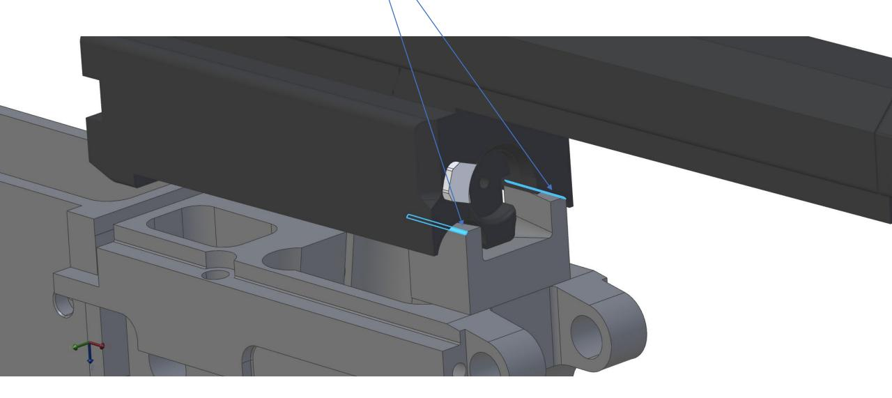
The blue areas show proper clearance needed on a feed ramp tower.
