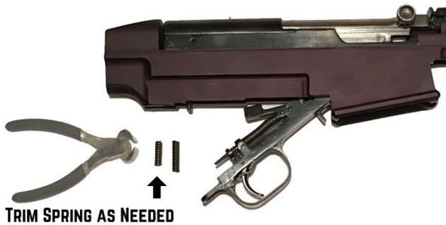
**Step 5.** Using the supplied spring, cut 1/8" from the spring. Install the trigger group the same way you would on a stock rifle. If the trigger does not snap into place (with a loud positive click) then pull the spring and reduce the height a further 1/8". You may need to do this several times in order to get a tight fit.
